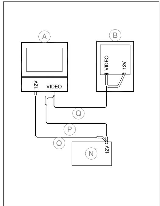
Fig. 3. Drawing of the receiving equipment. (A) Portable digital color recorder monitor (12 volts), (B) video receiver (12 volts), (N) 12 v battery, (O) Video recorder/monitor power cable, (P) Video receiver power cable, and (Q) Video transmission cable.
