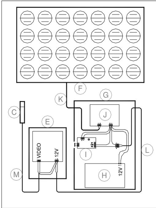
Fig. 2. Drawing of the transmitting equipment used to study Bearded Vulture breeding behavior. (C) Waterlight color microcamera (12 volts), (E) video transmitter (12 volts), (F) 75 W solar panel, (G) Battery charge control unit, (H) 12 volt, 12 amp battery, (I) Twilight switch (12 v), (J) Charge regulator, (K) Charge regulator power cable, (L) Video transmitter power cable, and (M) Power cable and video camera.
