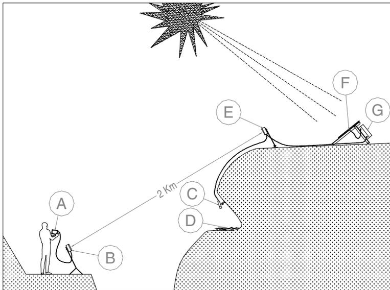
Fig. 1. Drawing of the video-monitoring system used to study Bearded Vulture breeding behavior. (A) Video recorder with a color monitor and battery, (B) Receiving antenna, (C) Camera, (D) Nest, (E) Transmitting antenna, (F) Solar panel, and (G) Power unit.
